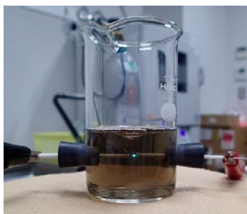
Figure 1. The photographic view of the experiment image synthesizing the Pd nanoparticles by the solution plasma method.
